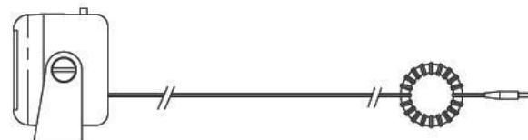
Figure 8. Power lead suppression.
