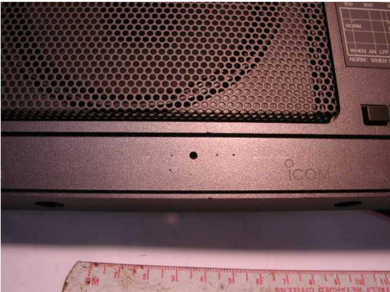
14. Notice the small indentations for the other three holes to be drilled. One on the left, two on the right.
