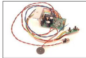
Above left: The DSP unit as supplied for in-speaker fitting.
