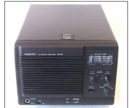
Right: The small DSP operation keypad is fitted to the speaker front panel (bottom, centre).
