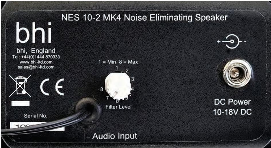
PHOTO 2: Rear view of the NES10-2 Mk4 showing the DSP control knob.
