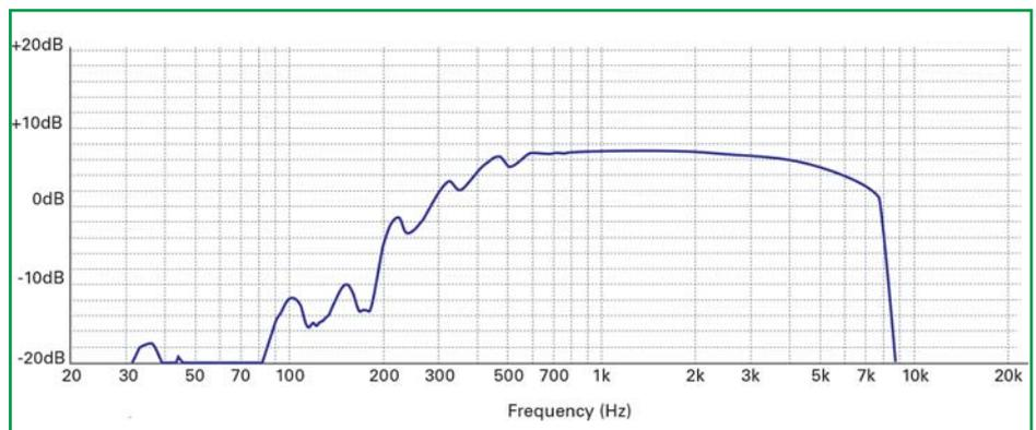
FIGURE 4: ParaPro EQ20 frequency response with the DSP noise filter set to mid-point.
